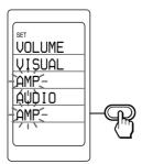
The component names are displayed on the labels. To change the labels, press the SCROLL button.
